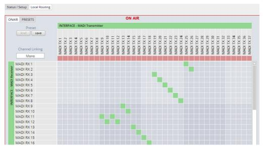
You can also assign device outputs (MAOUT 1 ... MDOUT 8) to MADI transmitter channels (MADITX 1 ... MADITX 8). For better visibility the matrix has been divided by cutting off the middle part:
