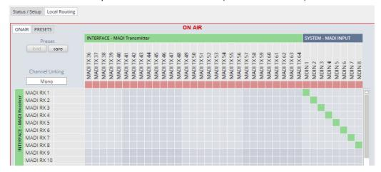
The **Local Routing** pane can also be used to route MADI signals from the receiver directly to the transmitter and vice versa:
