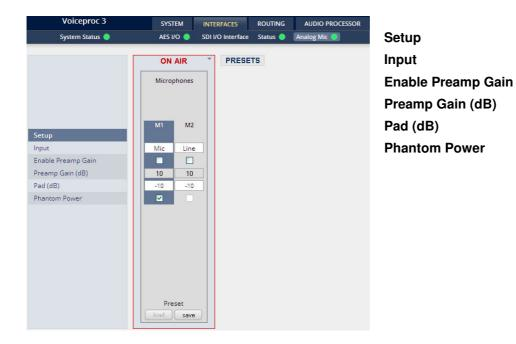
[Mic / Line] [ON / OFF] [10 ... 65] [OFF / -10] [ON / OFF] Phantom power is available when Input = Mic is selected.
