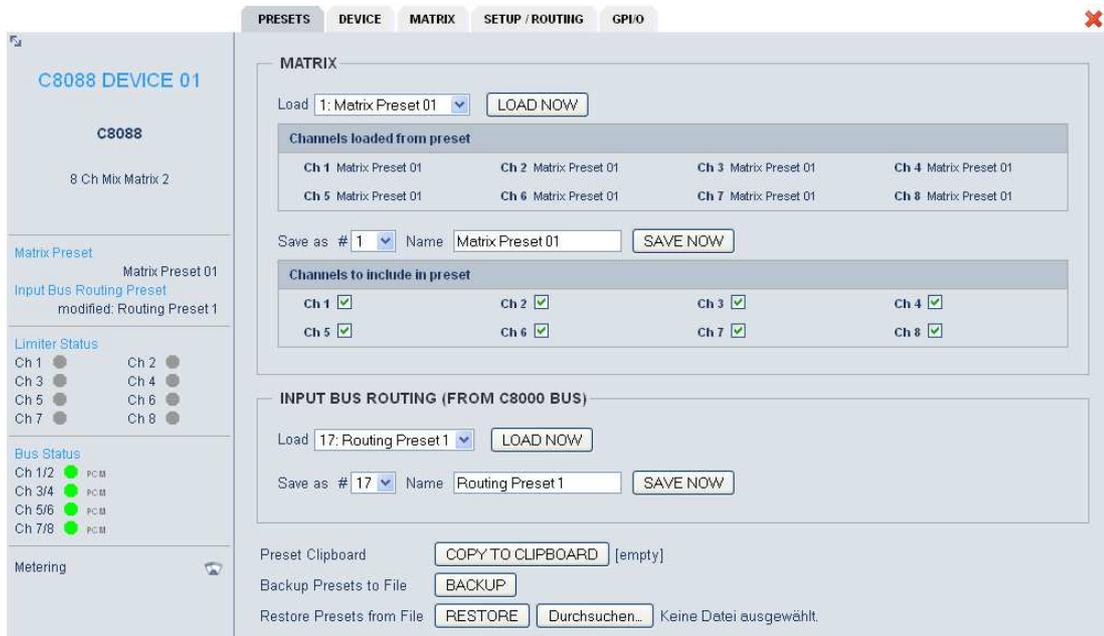
The **C8088** has **16 matrix presets** and **8 routing presets**. The status window at the left hand side shows the names of the active presets. The phrase “**modified**” will appear in line with the Preset name, if a preset parameter was changed by the operator.
