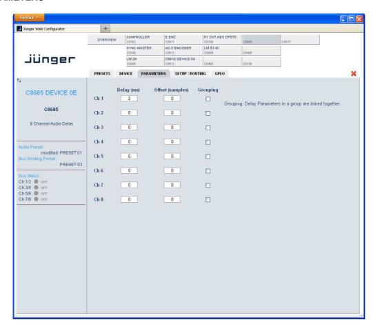
The display here depends on the Channel Mode selected on the SETUP / ROUTING pane. This example shows the delay configured for 8 independent channels.
