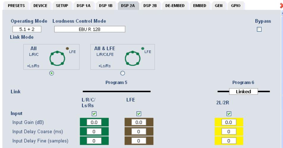
As mentioned above there is also a 5.1 + 2 program configuration available if you have bought the **surround option** for the C8492. In this case the first 6 channels of the DSP are linked for surround processing. This will also apply to **DSP 1** if 5.1 + 2 is selected. The example above shows a condition where the LFE is not linked to the other surround channels and may be controlled independently.
