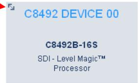
**C8492 DEVICE 00** - Given name of the module (may be changed on the DEVICE pane). It will be default set during initialization to module type amended by the word **DEVICE** and the CAN address **00** the module had at that moment.
