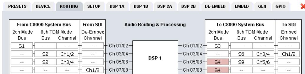
Similar applies to the output routing. [S3] is fed in 2Ch and [S6] in 8Ch mode. Duplicated busses [S4] are marked red as a warning because the signal will be disturbed if you connect two outputs to the same bus.
