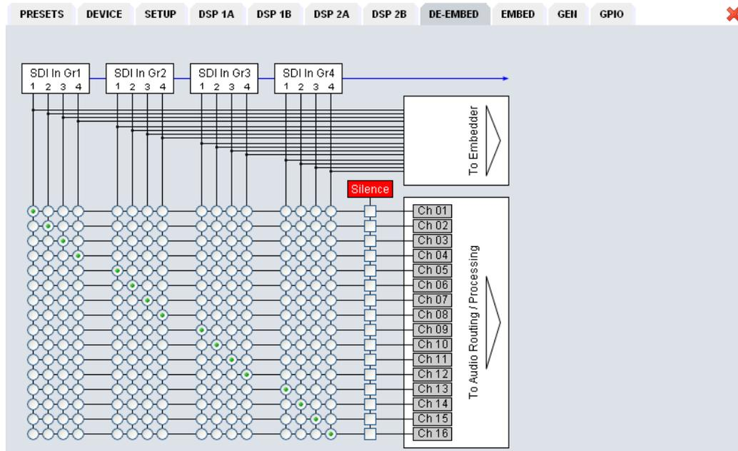
Here you may assign the audio signals from the 16 de-embedded channels to **up to 16** processing channels.
