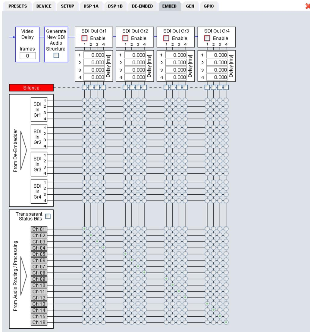
From here you can control the embedder. You may select between the 16 audio channels from the input (de-embedder) and the signals from the processors (DSPs).
