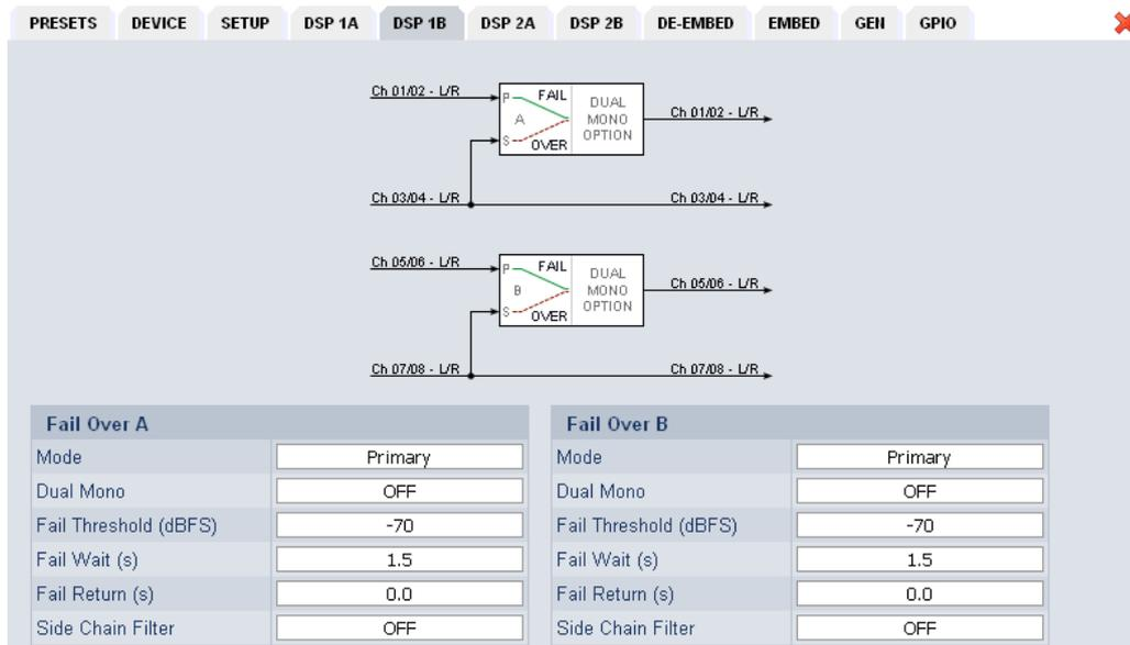
The **C8492** offers the feature to use pairs of channels in a fail over mode. I.e. if the audio signal fails in the first audio pair, the processor may switch over to the adjacent (e.g. 1/2 >> 3/4) pair automatically. The functions of the circuits Failover A – Failover B are similar. The switch over will be performed by a cross fade.
