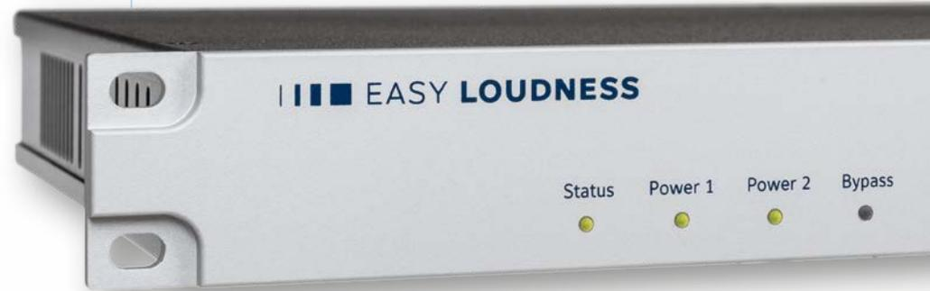
signal path, in case the main feed gets lost. The AES stereo input can be used as a fallback input if the SDI signal is interrupted.
