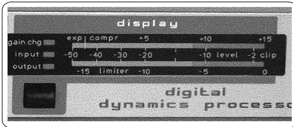
The two channel LED display has three display modes (input level, output level and gain change). Press the button in the display section to change the display mode. The selected display mode is indicated by the lighting of the appropriate LED above the display button and to the left of the display meters. For better visibility each display mode has its own LED colour and level meter colour.
