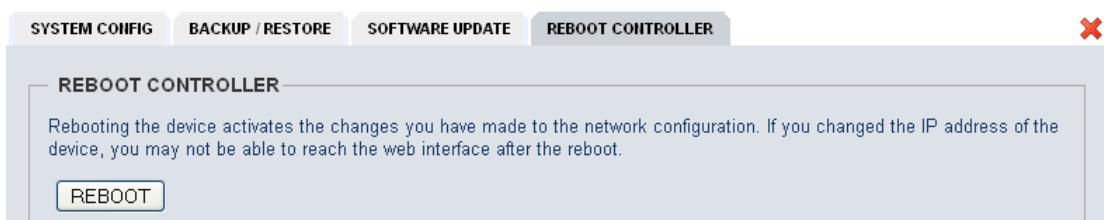
In order to make the IP configuration permanent you must reboot the frame controller.
