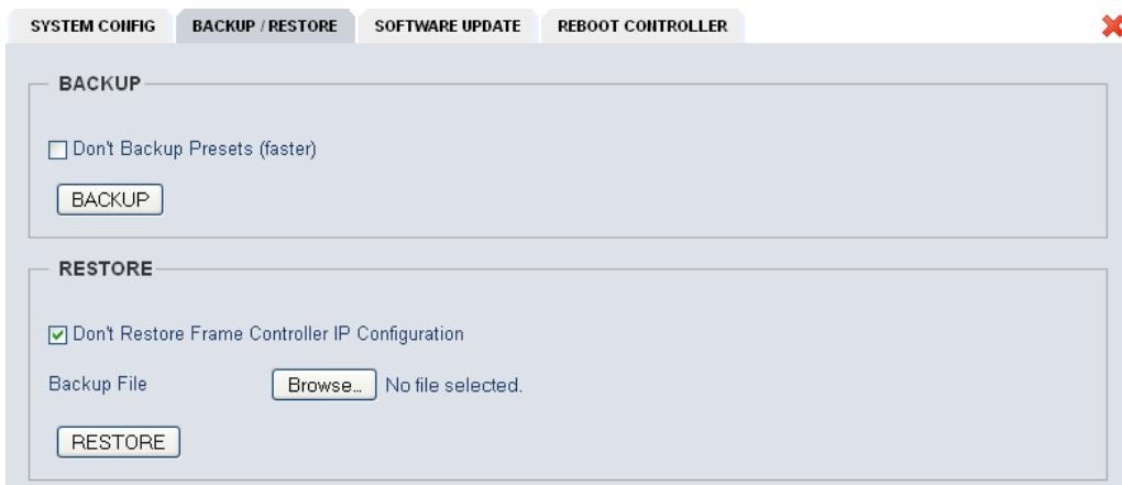
When you press <BACKUP> the frame controller will gather all information stored in individual modules of the frame and will build an **XML file** that contains such information. Due to the size of the frame and the complexity of the modules installed it may take a little while. When it's done you will be notified by a pop up. You must select "save file", press <OK> and a file dialog will open.
