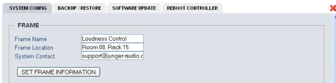
The **Frame Name** and the **Frame Location** as well as the **System Contact** are used by the SNMP **sysObject** OIDs (Object Identifier).
